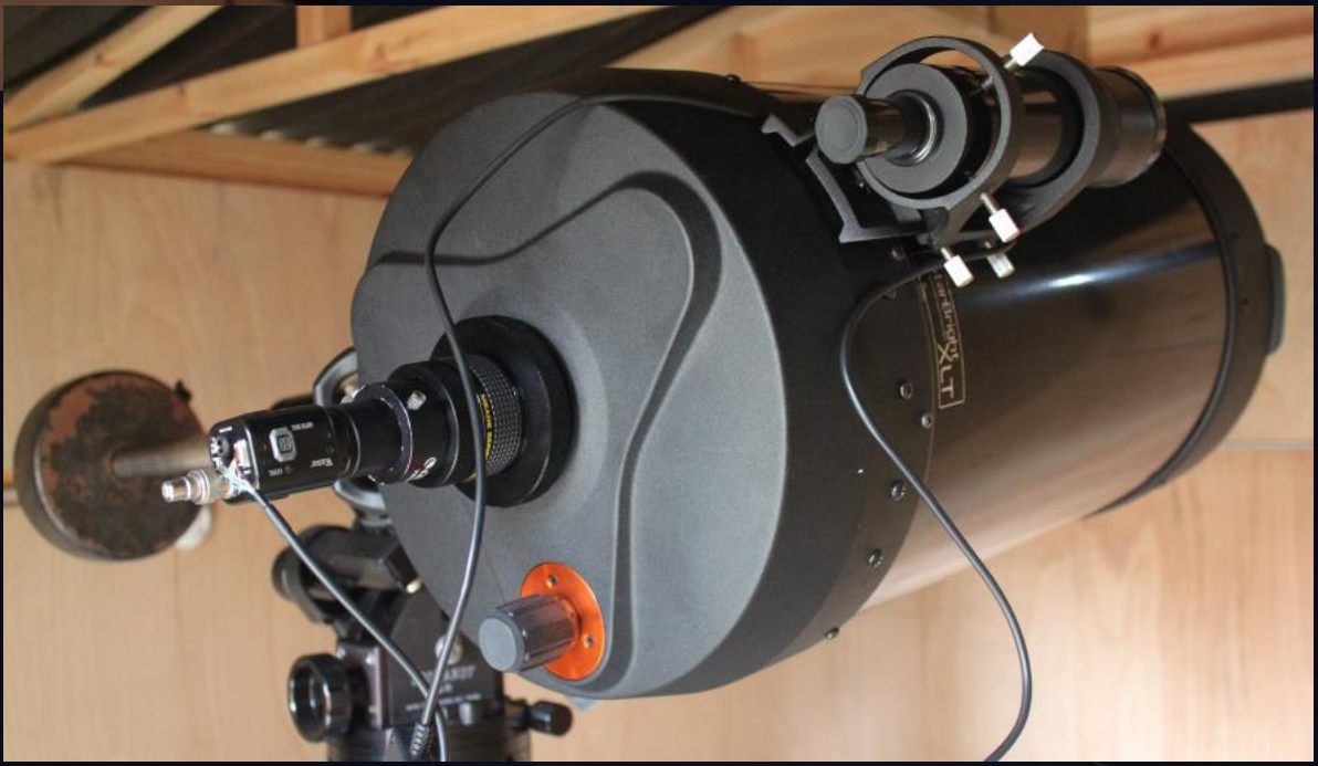
C11 f/10 @f/3.3 - Watec 910 – IOTA-VTI – Losmandy G11 mount and Gemini Go To
