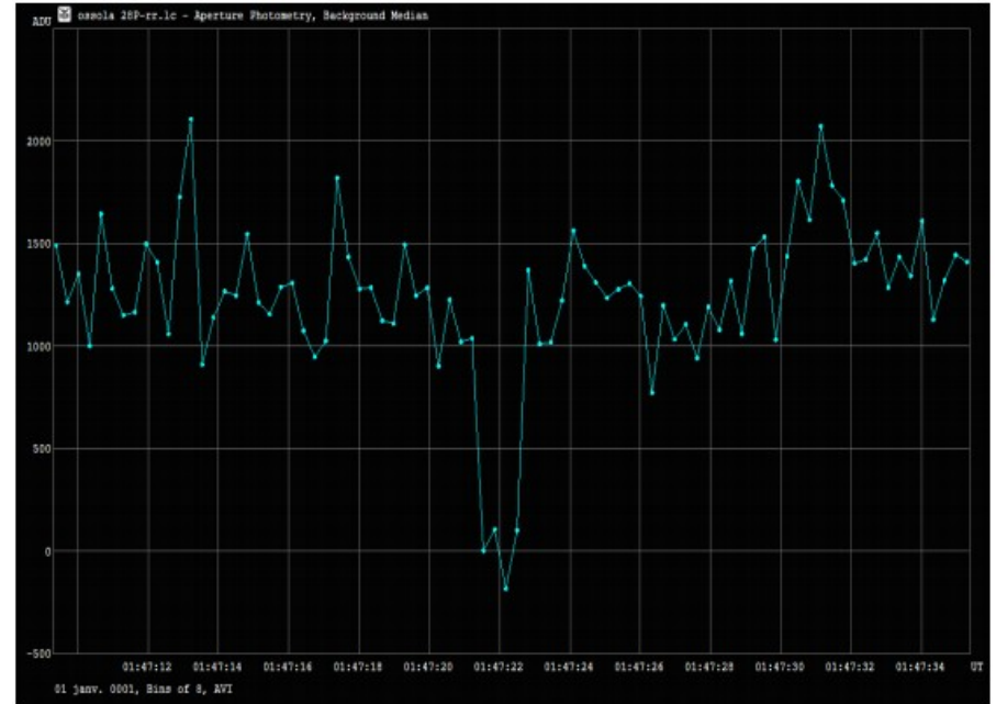
Figure 2. The lightcurve obtained by Alberto Ossola, Muzzano, Switzerland, 0.32 s integration time. Observed duration: 1.28 \pm 0.23 s, derived with Tangra.
